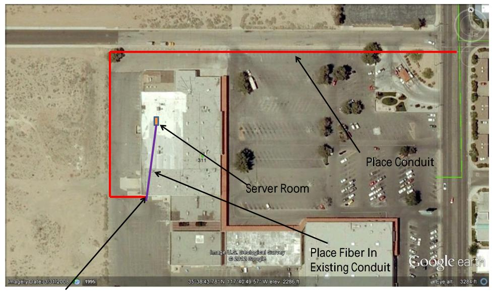
Penetrate Wall Here In Existing Hole With Conduit Caution Lead Paint On Outside Walls
